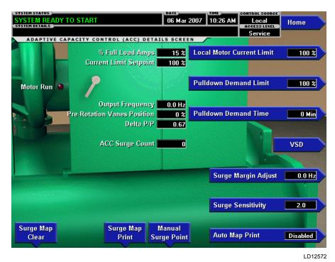
FIGURE 34 - ADAPTIVE CAPACITY CONTROL DETAILS SCREEN (SOFTWARE VERSION C.OPT.01.18.307 AND EARLIER) (VSD AND MV VSD)
