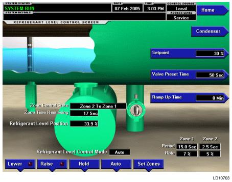
FIGURE 15 - REFRIGERANT LEVEL CONTROL SCREEN (SOFTWARE VERSIONS C.MLM.01.14.XXX AND LATER OR C.OPT.01.14.306 AND LATER)
