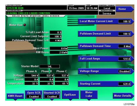
FIGURE 28 - MOD "B" SOLID STATE STARTER SCREEN
