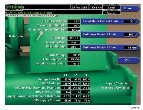
FIGURE 39 - HARMONIC FILTER DETAILS SCREEN (STYLE D VSD AND VSD WITH PART NUMBER 371-03789-XXX (503HP 60HZ; 419HP 50HZ)
