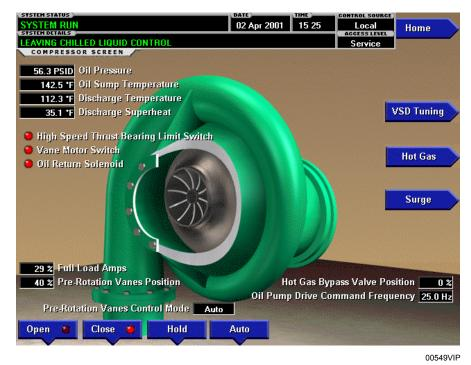
FIGURE 16 - COMPRESSOR SCREEN (ALL "P" COMPRESSORS AND STYLE F AND LATER CHILLERS WITH G, Q OR H5-8 COMPRESSORS)
