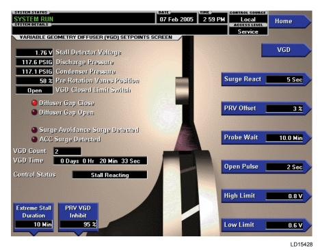
FIGURE 22 - VARIABLE GEOMETRY DIFFUSER SETPOINTS SCREEN
