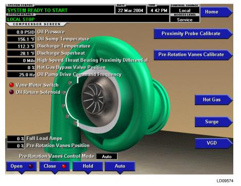
FIGURE 17 - COMPRESSOR SCREEN (STYLE E AND EARLIER CHILLERS WITH G, H, OR J COMPRESSORS AND STYLE G CHILLERS WITH K COMPRESSORS)
