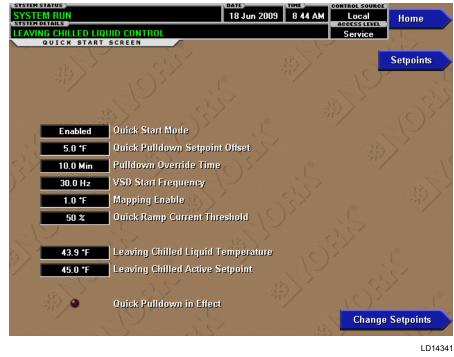
FIGURE 45 - QUICK START SCREEN (SOFTWARE VERSION C.OPT.01.21.307 AND LATER)
