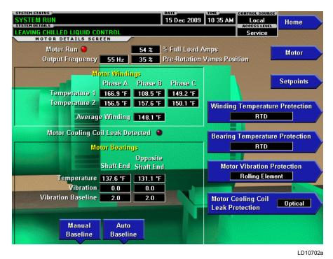
FIGURE 41 - MOTOR DETAILS SCREEN (SOFTWARE VERSION C.OPT.01.22.307 AND LATER)
