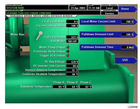
FIGURE 32 - VARIABLE SPEED DRIVE (VSD) DETAILS SCREEN (STYLE D VSD AND VSD WITH PART NUMBER 371-03789-XXX (503 HP 60HZ; 410HP 50HZ))
