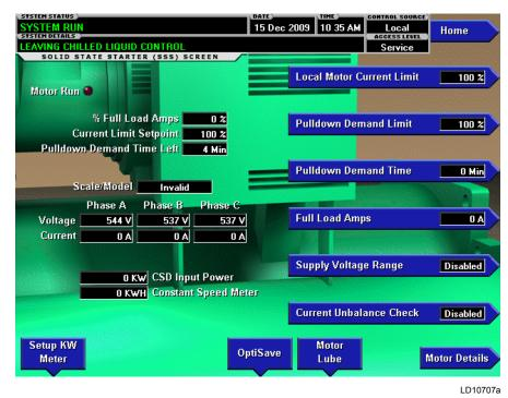
FIGURE 27 - MOD "A" SOLID STATE STARTER SCREEN
