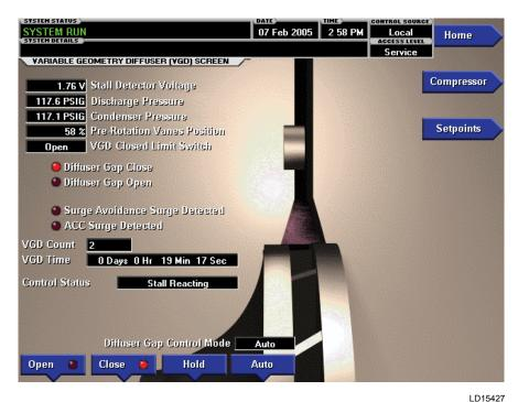
FIGURE 21 - VARIABLE GEOMETRY DIFFUSER SCREEN
