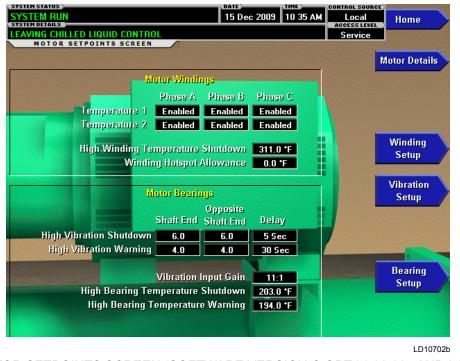
FIGURE 42 - MOTOR SETPOINTS SCREEN (SOFTWARE VERSION C.OPT.01.22.307 AND LATER)
