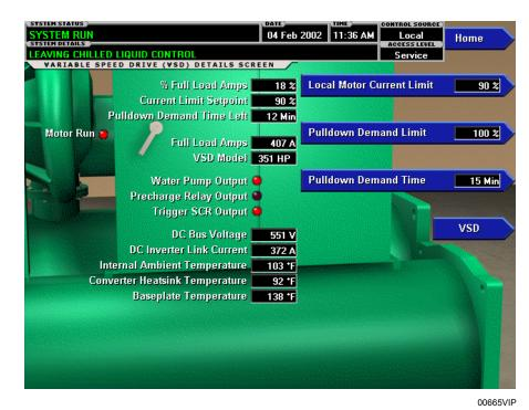
FIGURE 33 - VARIABLE SPEED DRIVE (VSD) DETAILS SCREEN (VSD WITH PART NUMBER 371-02767-XXX (60HZ) OR 371-03700-XXX (50HZ))
