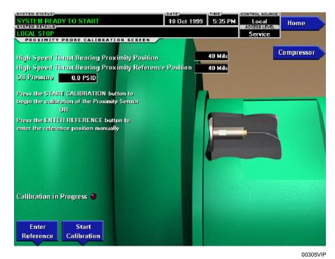
FIGURE 18 - PROXIMITY PROBE CALIBRATION SCREEN (STYLE E AND EARLIER CHILLERS WITH G, H, OR J COMPRESSORS AND STYLE F AND LATER CHILLERS WITH J OR H3 COMPRESSORS)
