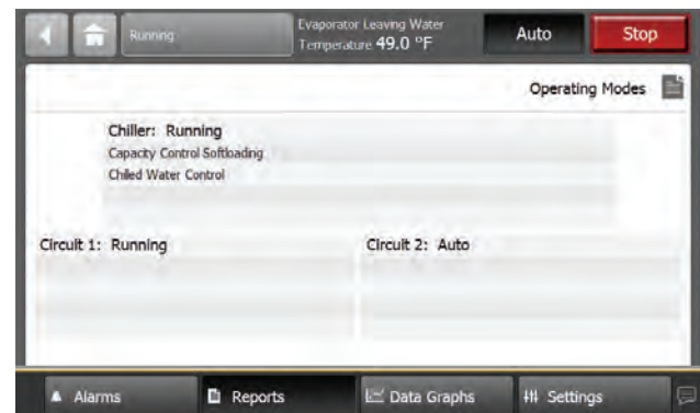
Figure 29. Chiller operating modes
