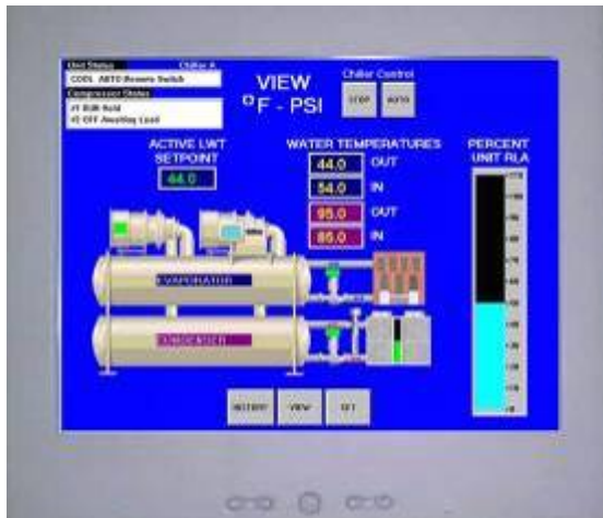
Figure 22, MicroTech II Control Panel
