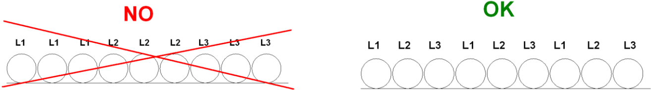
Fig. 1 - Installation of long power supply wires
