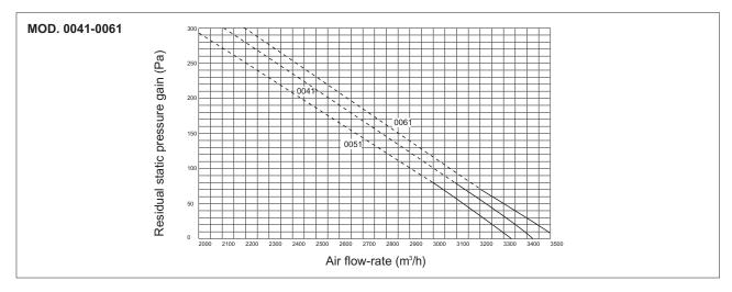
⚠ The characteristics indicated above refer to units with ducted outlets, with a 0.5m long straight duct and a cross-section equal to the cross-section of the fan.
