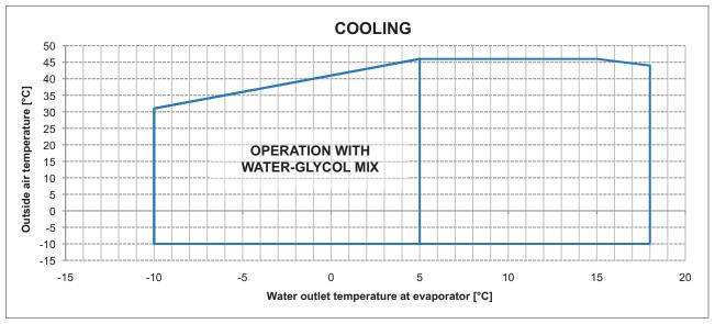
Operating range in COOLING Water temperature head min-max= 3-8 K Water circuit pressure min-max= 1÷6 bars Max storage temperature= 63°C Maximum percentage of glycol= 40%
