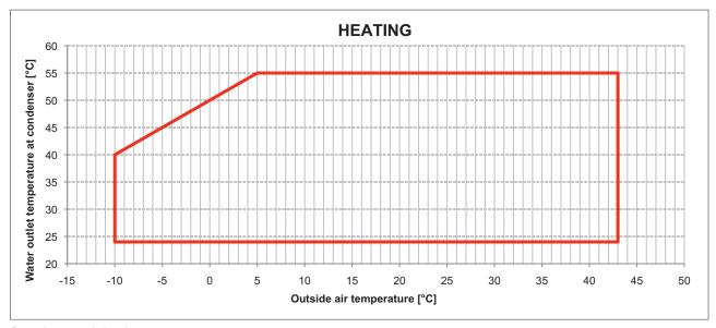
Operating range in heating Water temperature head min-max= 4-10 K Water circuit pressure min-max= 1÷6 bars Maximum water temperature at system heat exchanger water inlet +50°C Max storage temperature= 63°C Maximum percentage of glycol= 40%
