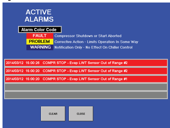
Figure 52: Active Alarms Screen
