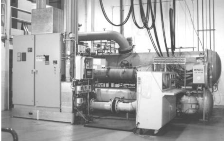
McQuay's new million dollar compressor test stand with state-of-the-art data acquisition provides comprehensive information on new compressor designs.
