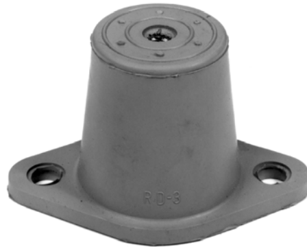
TYPE R OR RD IF BOLTING IS PREFERRED— Type R or RD mountings are furnished with a tapped hole in the center. This enables the equipment to be bolted securely to the mounting.
